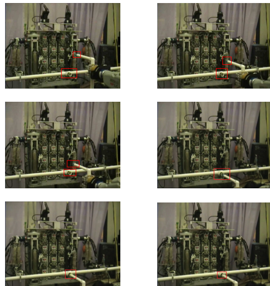
Fig. 2. Experiment 6: Two heterogeneous robots cooperate to perform a joint assembly using force sensing under a push-push coordination scheme.
